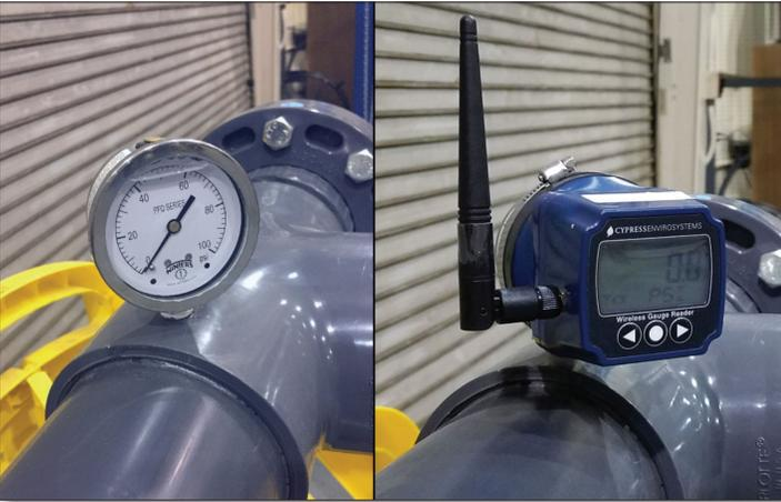
Figure 14 – WGR installed on pressure gauge
