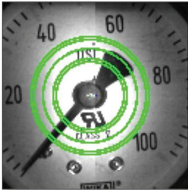
Figure 13 – Properly set-up concentric circles
