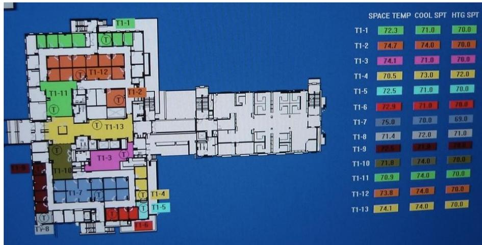
Figure 5: Pilot Site 1 - Thermostat Deadband Setpoints
