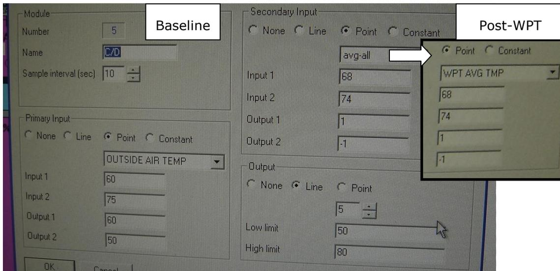
Figure 4: Pilot Site 1- CD SAT Reset Baseline (main) and CD SAT Rest Post-WPT (insert):
