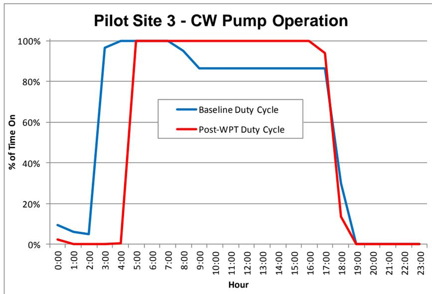
Figure 26: Pilot Site 3 – Condenser Water Pump Operation
