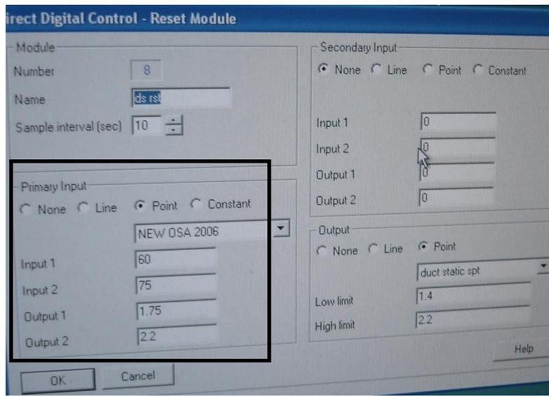
Figure 11: Pilot Site 1- DSP Reset based on OAT, not Zone Information
