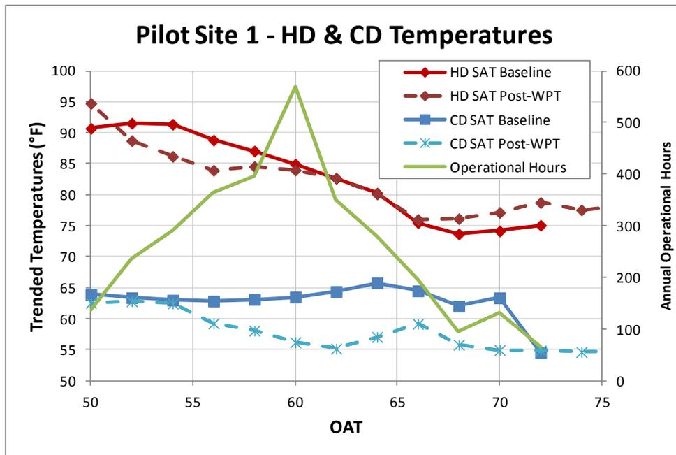
**Figure 10: Pilot Site 1 - Hot Deck and Cold Deck Temperatures Trends**
