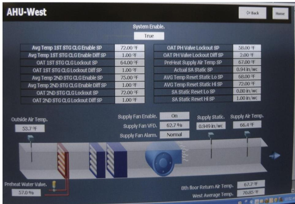
Figure 16: Pilot Site 2 - Cooling Stage Lockout based on OAT and Average Building Temperature
