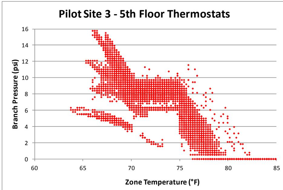
Figure 23: Pilot Site 3 - 5<sup>th</sup> floor Zone Temperature versus Branch Pressure
