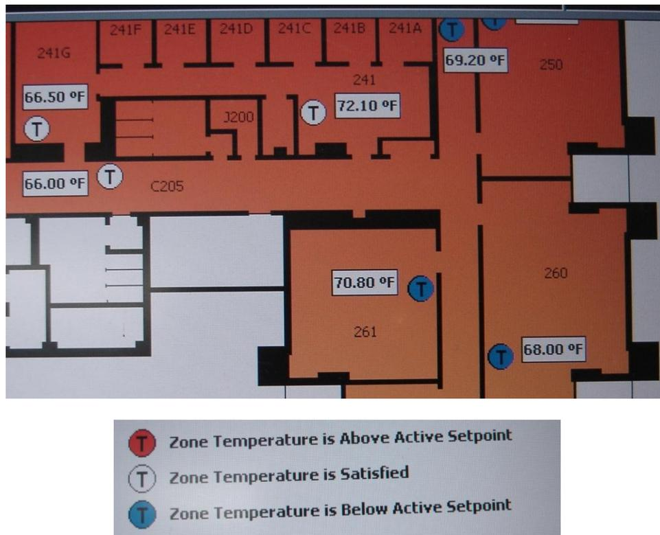
Figure 34: Pilot Site 4 – Detail of 2<sup>nd</sup> Floor BMS Screen (top) and Thermostat Color Key (bottom)
