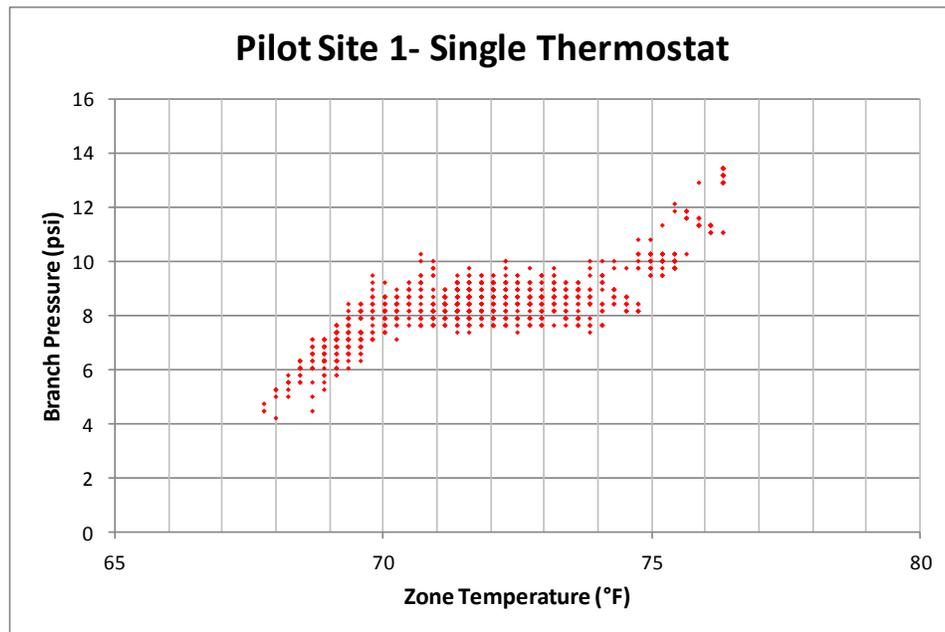
Figure 6: Pilot Site 1- Branch Pressure versus Zone Temperature, single zone
