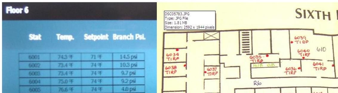
Figure 37: BMS List of WPTs by Floor (left) and Hard-Copy Map of WPT Locations (right)
