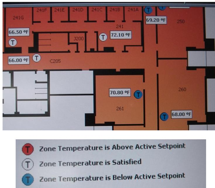
Figure 38: Example of Zone Map with Color-Coded Thermostats (above) and Key (below)
