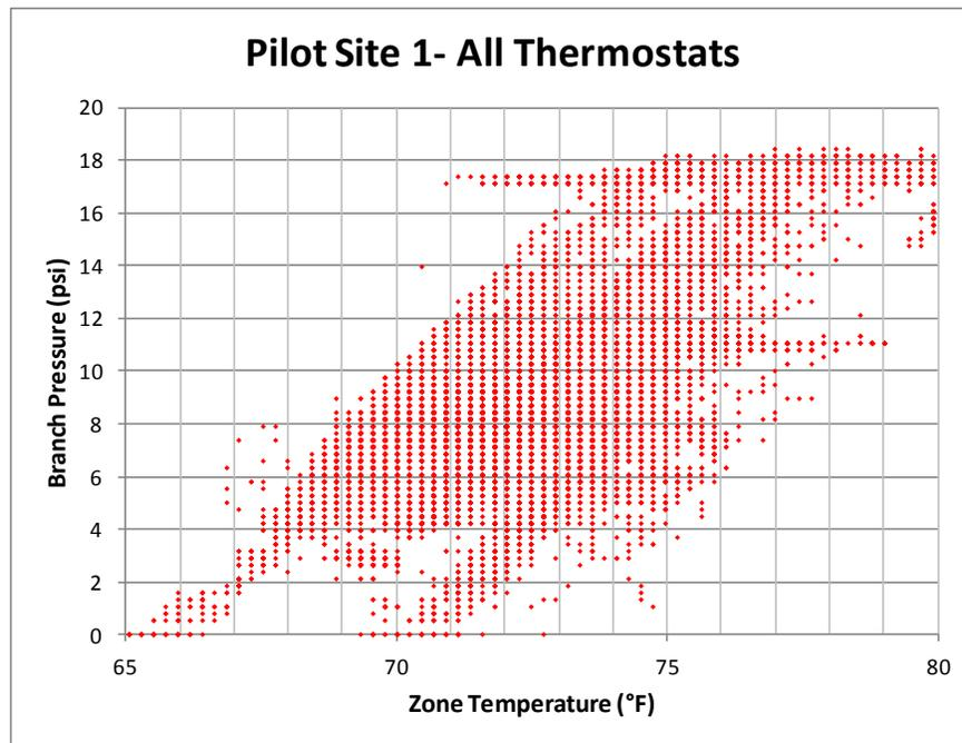
Figure 7: Pilot Site 1- Branch Pressure versus Zone Temperature, all zones
