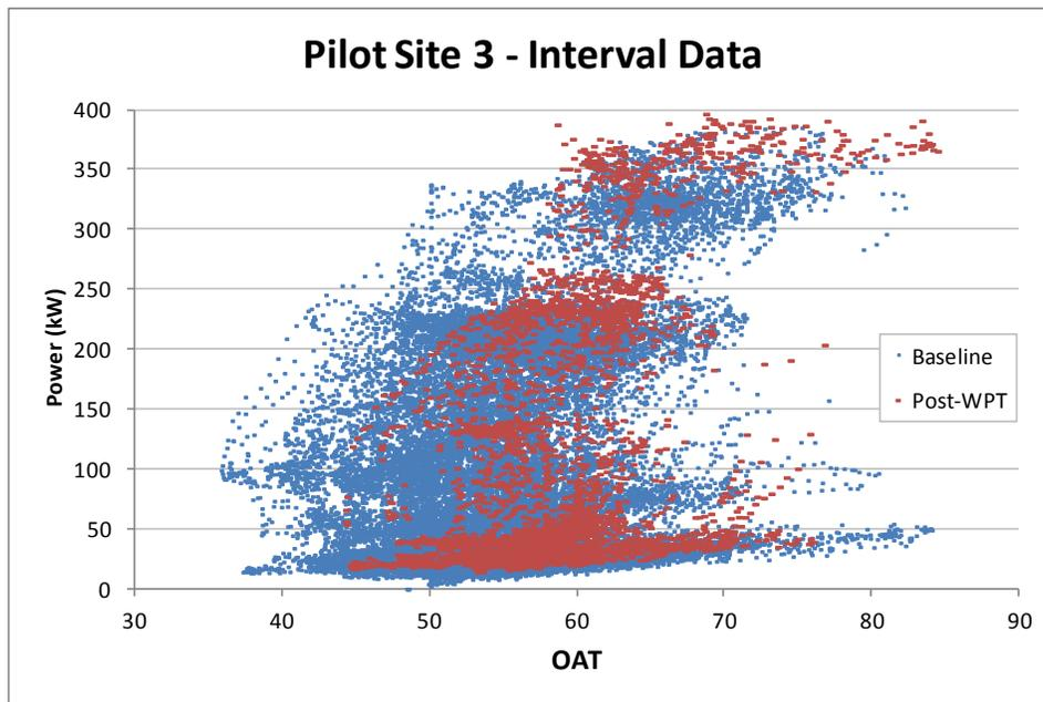
Figure 24: Pilot Site 3 - Building Operating Power versus OAT
