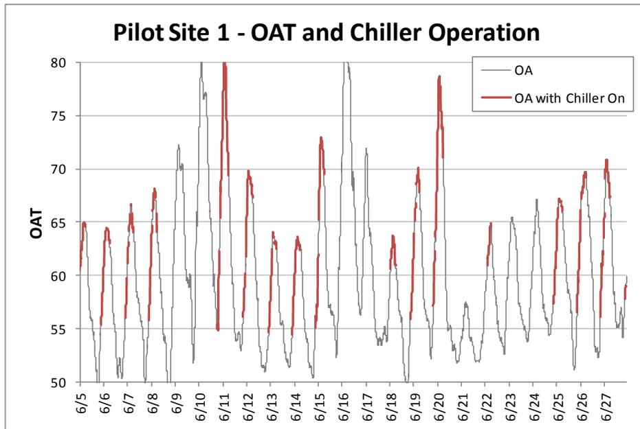
Figure 13: Pilot Site 1– Cycling Chiller Operation
