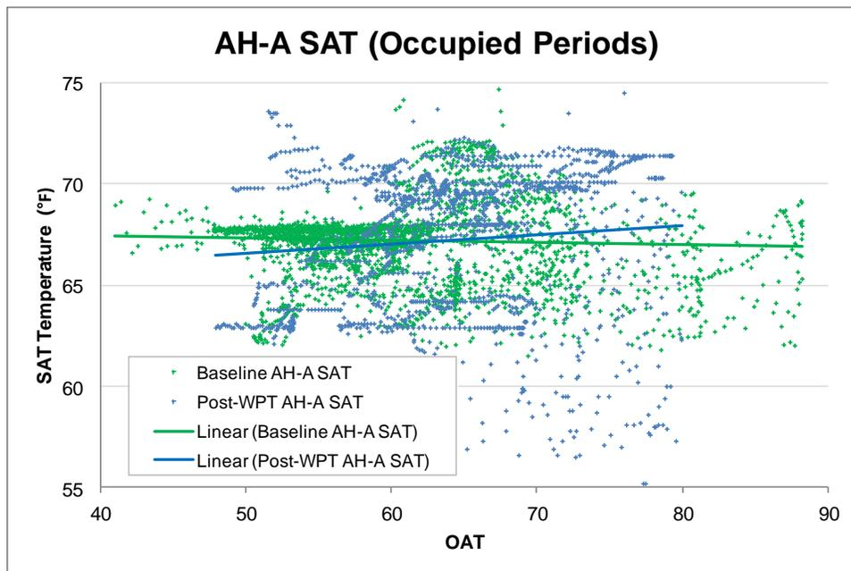
Figure 30: Pilot Site 4 – Measured SAT Before and After WPT Retrofit
