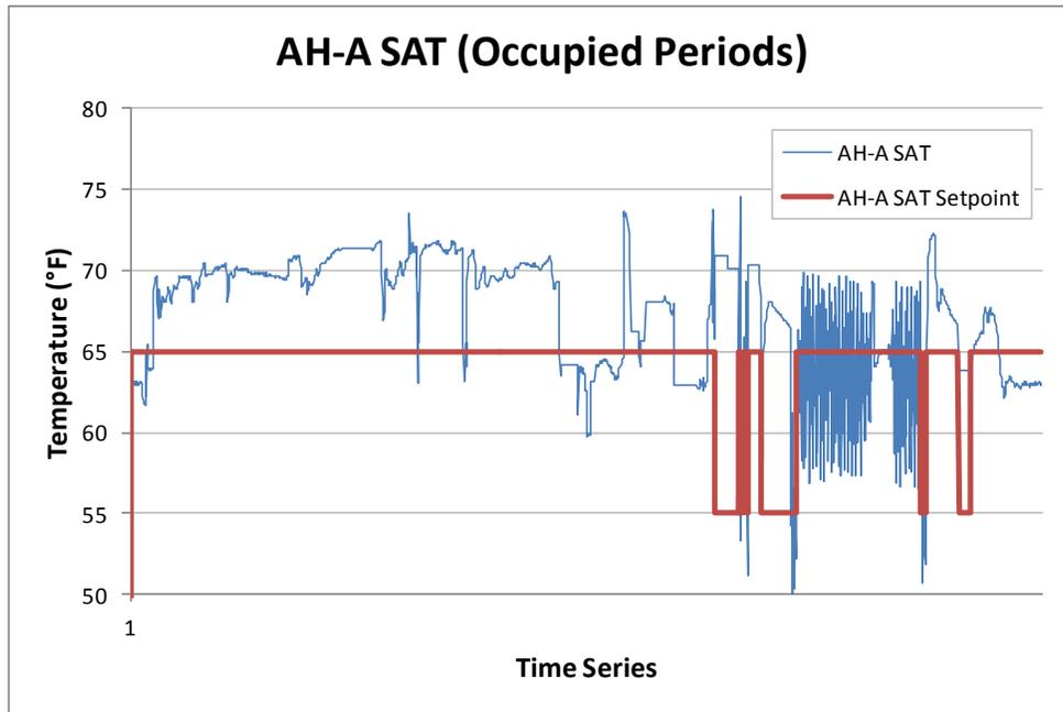
Figure 29: Pilot Site 4 – SAT Setpoint and Measures Temperature After WPT Retrofit, Occupied Times
