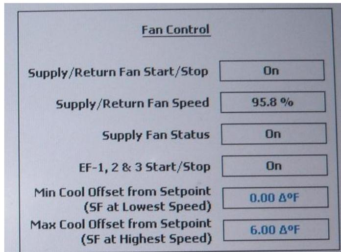
Figure 32: Pilot Site 4 – Fan Speed Control at the End of the Post-WPT Monitoring Period
