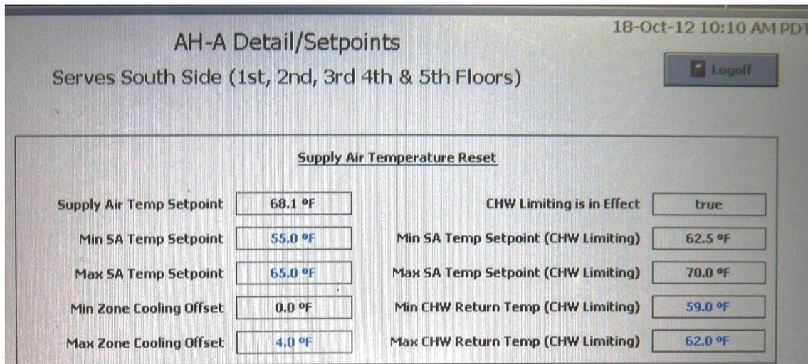
Figure 27: Pilot Site 4 – SAT Control Screen at the Start of the Post-WPT Monitoring Period
