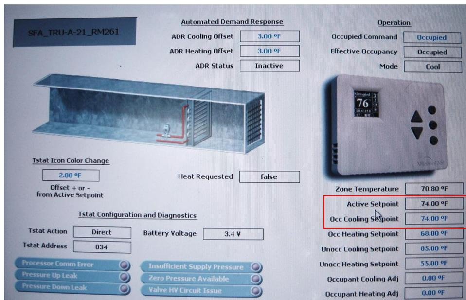
Figure 33: Pilot Site 4 – Deadband Visible in Zone Graphic
