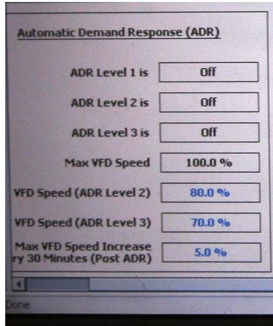
Figure 36: Pilot Site 4 – Demand Response Fan Speed Control
