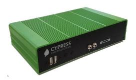
Network and Data Controller for Cypress Envirosystems WPT networks. Use to make data available to existing building automation systems, or use standalone with the WPT Web interface.
