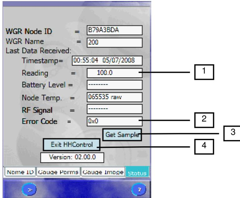
1. **Reading:** Contains reading results from a Get Sample Request. This is used to verify the calibration of the WGR was accurate.
