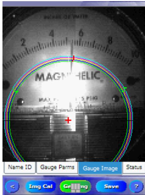
Notice also the Red Pixels in the images above. They represent the needle location determined by the WMR image processing algorithm. The Red Pixels behave the same for a Get Sample as they did for regular gauges.
