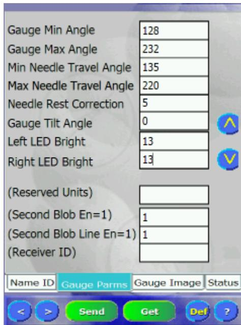
If you notice a contrast difference running down the middle of the image, the left and right half do not match in brightness. To adjust the brightness the **Left and Right LED Bright** variables need to be adjusted. Decreasing the value will make the image darker; increasing the value will make the image brighter.
