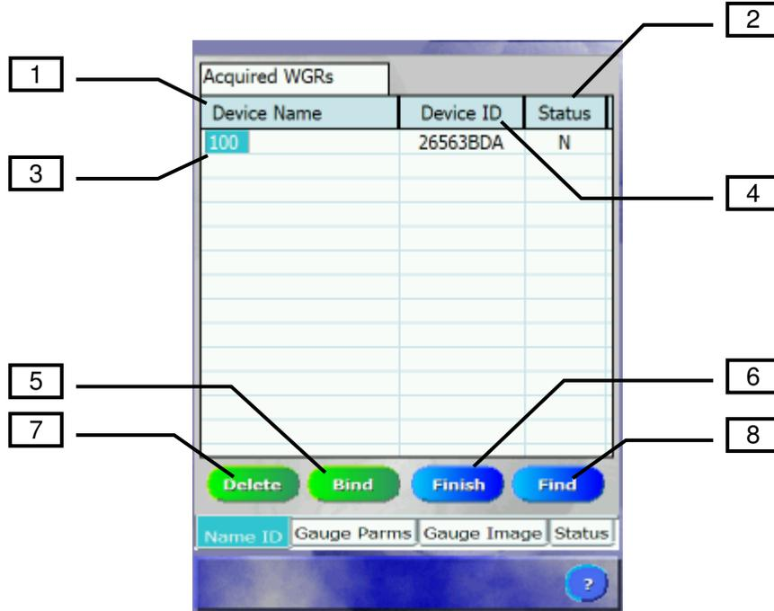
1. **Device Name Column:** This column contains the name of the WGR that the handheld is or has bound to. This is used to identify the WGR by name. Highlighting a WGR from the list will recall its parameters from the saved text file.
