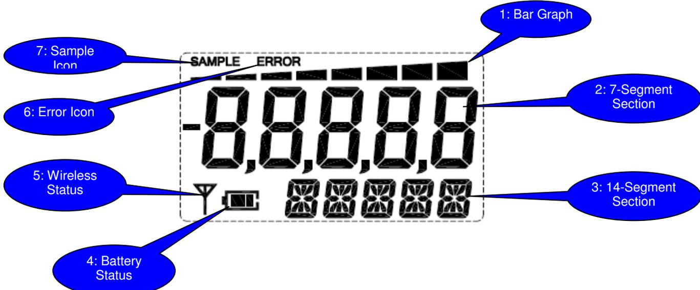
1. **Bar Graph:** This graph is a visual representation of the latest gauge reading. The graph grows from zero to eight bars as the needle moves from its minimum to maximum position.
