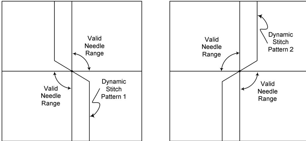
Figure 4: The possible needle angles for each pattern.
