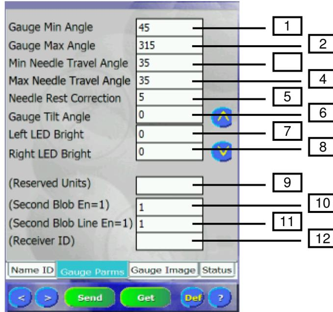
1. **Gauge Min Angle:** Angle, with respect to Gauge Bottom, at which the Min Gauge Value resides.
