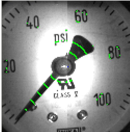
Here is an example of concentric circles properly setup. It may be impossible to avoid all background markings but you must attempt to minimize them. The image processing algorithm will ignore the numbers, rivets and the large graphic in this example. However, portions of the PSI symbol and the top of the “100” marker are still overlapped. The algorithm includes processing steps to filter out as much noise as it can, so a certain amount is tolerable.
