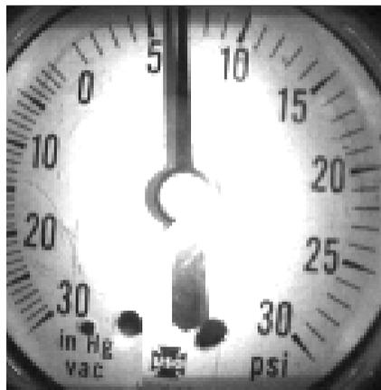
Figure 6: Glare from the left LED on the bottom of needle.
