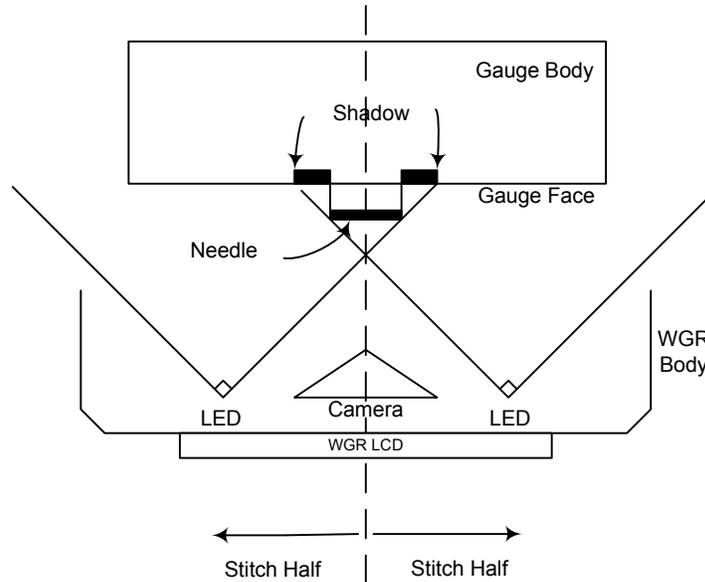
Figure 1: Illustration of Stitching two halves of an image using two LEDs.
