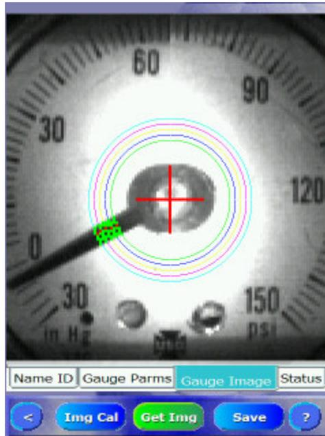
For a No Tip Needle, do the same as a No Tail. To reverse the readings you must rotate the Gauge Min, Gauge Max, and Min/Max Needle Travel Angle by 180 degrees in your setup.
