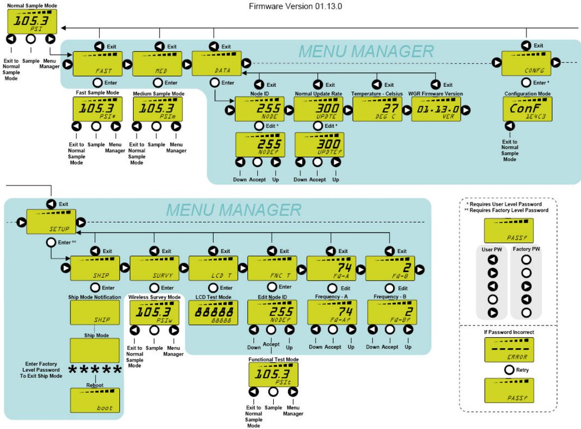
1. **Normal Sample Mode:** When the WGR is not in any special operating mode it is in the Normal Sample Mode. In this mode the WGR will periodically wake up, sample the gauge, transmit the reading, and update the 7-segement section on the LCD to the most recent value. The time between samples is setup using the HH.
