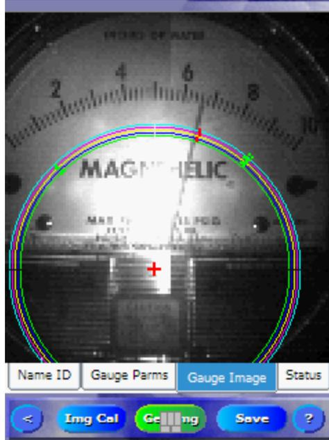
This is an example image that shows the Arcs in the wrong location. Notice the needle can travel past the end of the Arcs. When the needle is beyond the end of the Arcs, they will not be processed and an error will be sent. The Min and Max Needle Travel Angles for this example are shown below, 135° and 220° respectively.
