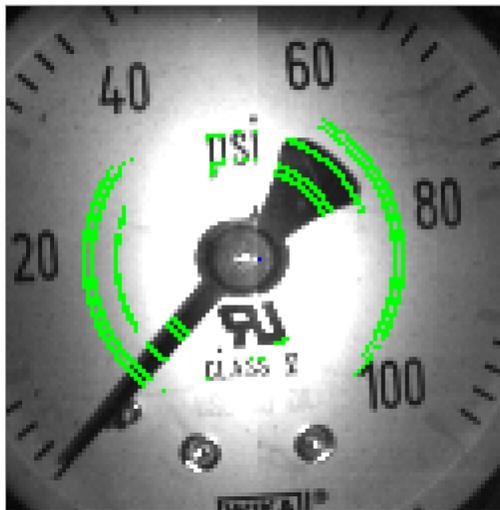
Here is an example of when the Pixel Threshold needs to be decreased. Notice the entire needle is not being picked up.
