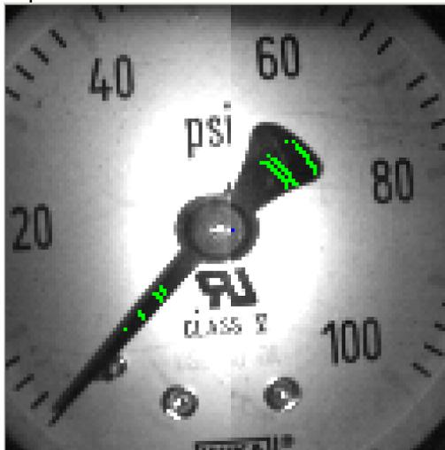
To ensure a robust setup we must set the Pixel Threshold so it is not at the edge of picking or dropping extra pixels. The camera exposure and lighting can vary depending on
