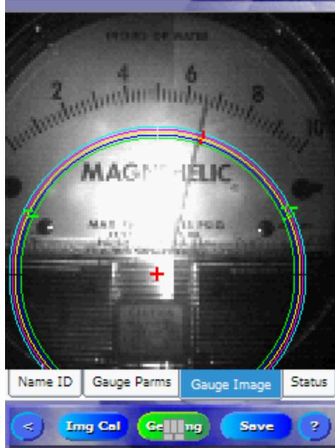
The image above shows the Arcs end in the proper location. You do not want them to overlap the Needle Stops or the black circles at the ends. The Min and Max Needle Travel Angles for this example are shown below, 115° and 245° respectively.
