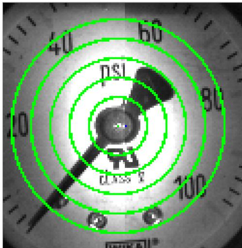
The image below is the same as the one above except the green pixels represent what the image processing algorithm considers the needle. Notice all green pixels outside of the needle. These could confuse the image processing algorithm and distort the reading.
