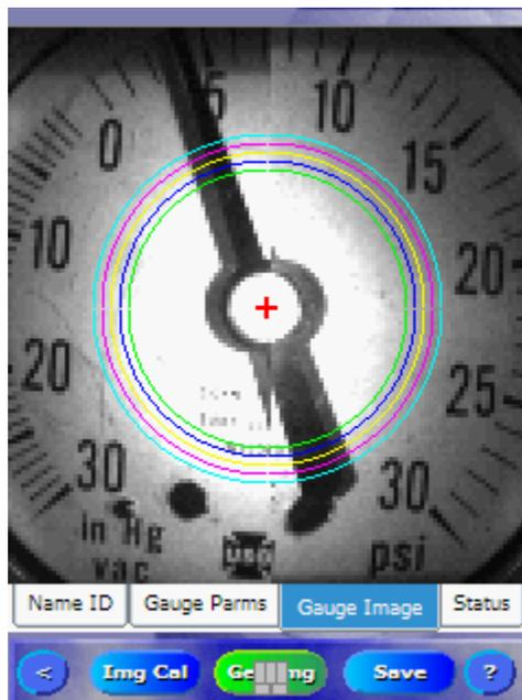
3. If Zoom is enabled, set the Zoom X and Y Offset to  $[63 - \text{Center Point X/Y}]$ , and set Center Point X and Y to 63. See the Circle Calibration section.
