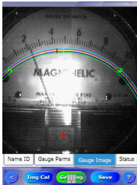
To get around this problem we recommend configuring the circles as seen in the image below. In this case, the Arcs stop passed the needle stops. If a needle were resting on the stops they would be processed.
