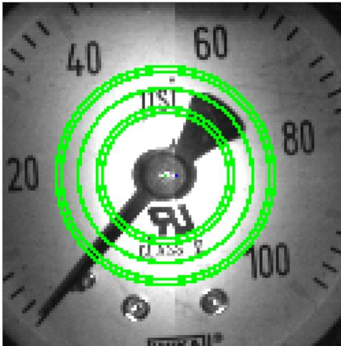
The image below is the same as the one above except the green pixels represent what the image processing algorithm considers the needle. This result is much better than the previous example. The majority of the green pixels are concentrated only on the needle.
