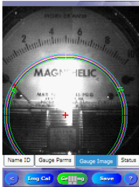
The **Center Point X** of the circle should match the center of the Gauge Face. The **Center Point Y** of the circle should be adjusted as needed such that the circles are properly spaced between the needle stops and the Magnehelic text.
