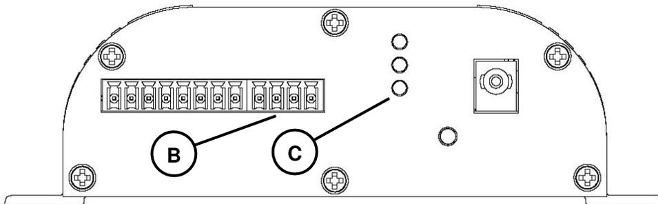
4. After normal start up note the special Calibration Successful sequence on the three LEDs (C). If the calibration was successful all three LEDs (Red, Orange, and Green) will blink quickly 3-times in a row.
