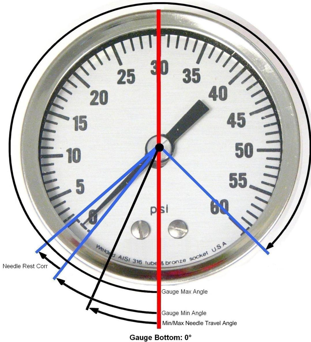
Often a gauge is installed at an angle. It makes sense to mount the WGR right side up for readability. It is also possible that a WGR must be mounted at angle if obstacles exist. In either case the WGR must be setup with the correct tilt angle between itself and the gauge.
