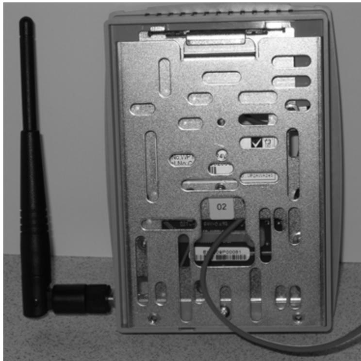
**Figure 7. Wall Bracket Cable Routing Recommendation**
