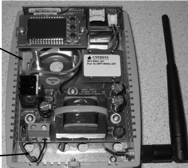
**Figure 6. Internal Cable Routing Recommendation**
