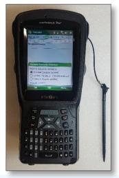
Figure 9 – WGR calibration tool
