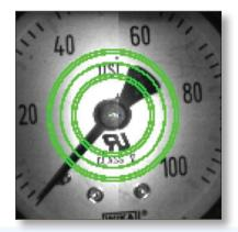
Figure 13 – Properly set-up concentric circles
