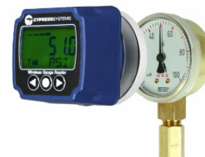
Wireless Readers Mounts Over Existing Gauges
