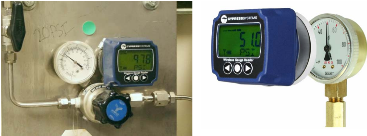
Figure 2 – Non-Invasive Mounting for Wireless Gauge Reader
