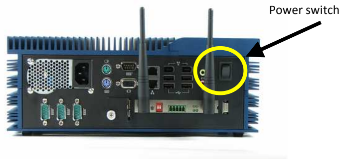
Figure 3. BBS Power Switch Location
