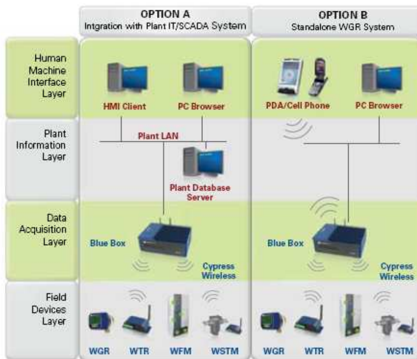
Figure 2. Cypress Envirosystems Monitoring System Setup Options
