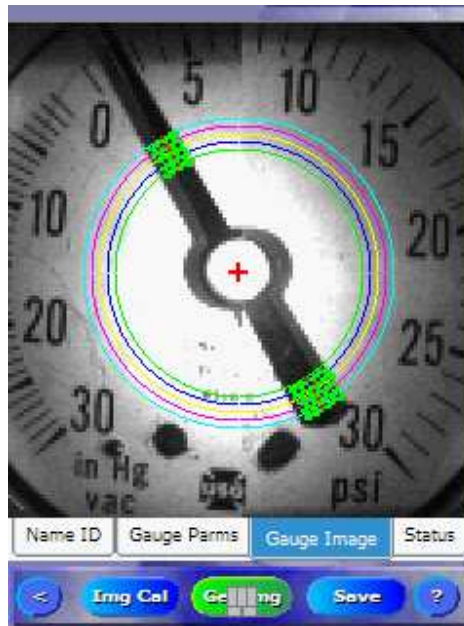
Figure 35. Green and Red Pixels Superimposed on the Gauge Image
