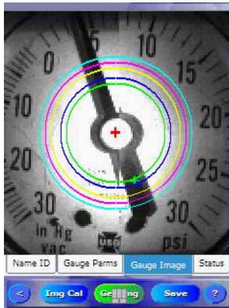
Figure 33. Radii and Center Point Calibration
