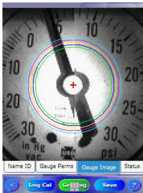
Figure 34. Radii and Center Point Calibration
