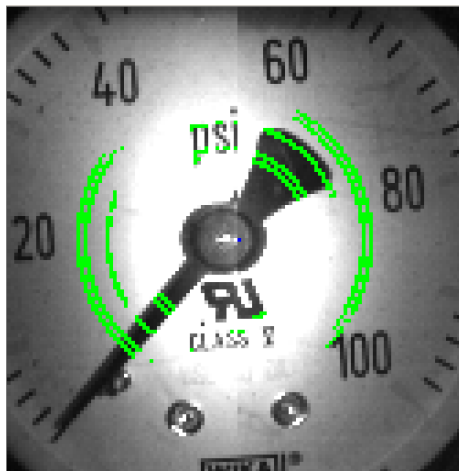
Figure 20. Pixel Threshold Adjustment Required - Increase
