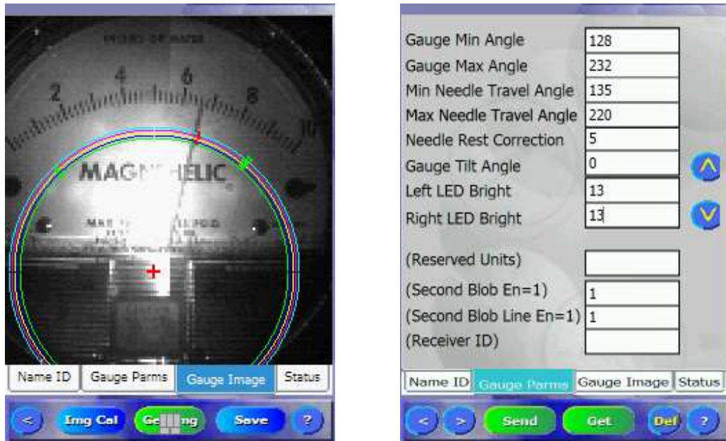
Figure 46. Improper Circle Setup
