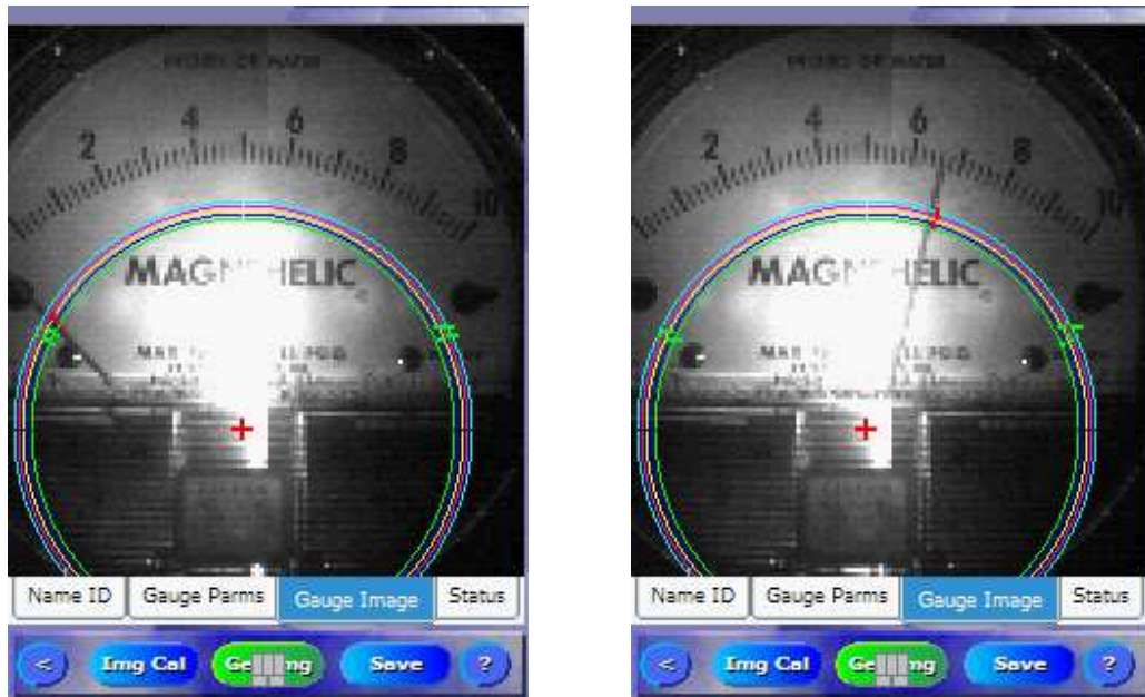
Figure 44. Proper Circle Setup for the WGR on a Magnehelic gauge
