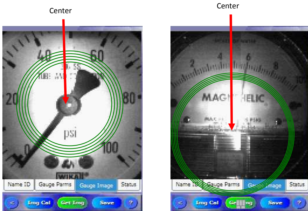
Figure 37. Circles for a Traditional Gauge versus a Magnehelic Gauge
