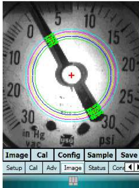
Figure 37 : Green and Red Pixels Superimposed on Image
