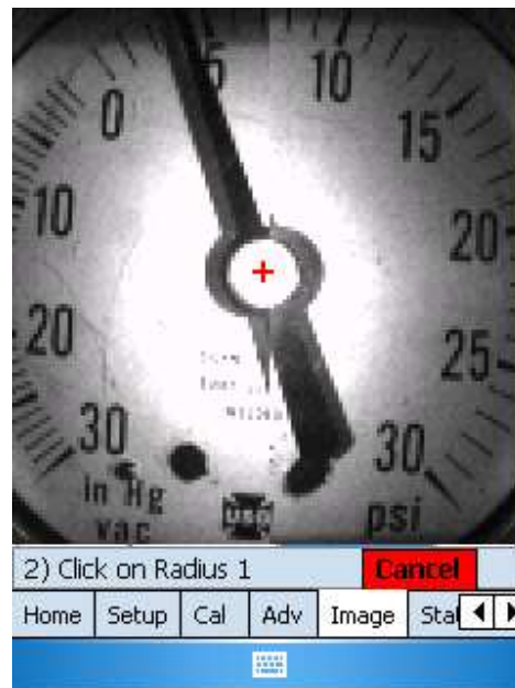
Figure 35 : Gauge Center Calibration
