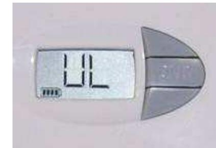
**NOTE:** The LCD buttons can also be locked/unlocked from the WPT Green Box.
