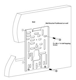
Figure 5. Mounting the Universal Wall Bracket
