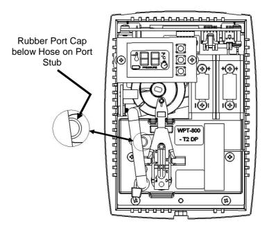
Figure 18. 2 Pipe Thermostat Port Cap
