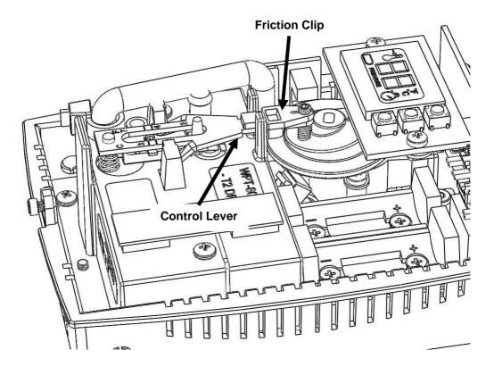
Figure 15. Friction Clip and Control Lever
