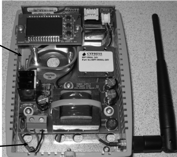
Figure 6. Internal Cable Routing Recommendation
