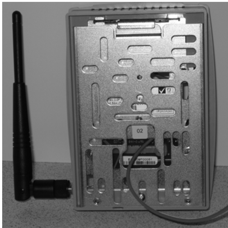
Figure 7. Wall Bracket Cable Routing Recommendation
