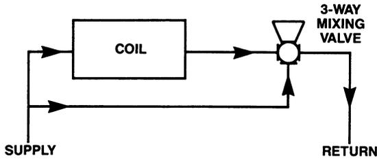
**COIL BYPASS USING THREE-WAY VALVE
