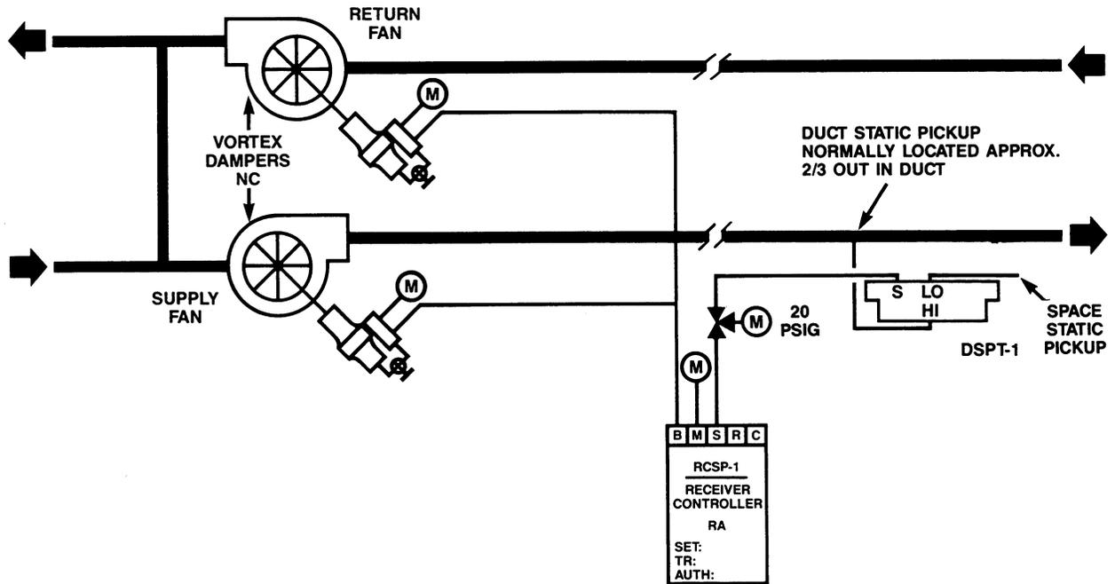
OPEN LOOP SUPPLY AND RETURN FAN CAPACITY CONTROL
