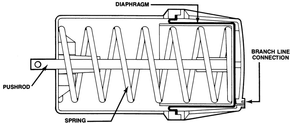
CUTAWAY OF DAMPER ACTUATOR
