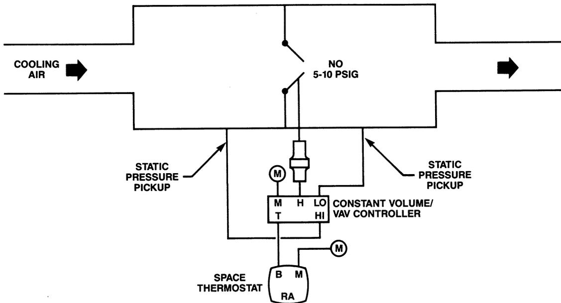
VAV TERMINAL UNIT WITH HIGH LIMIT
