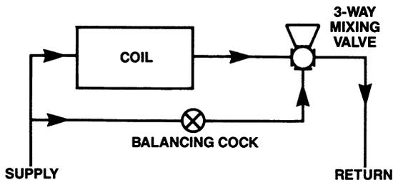
**COIL BYPASS WITH BALANCING COCK
