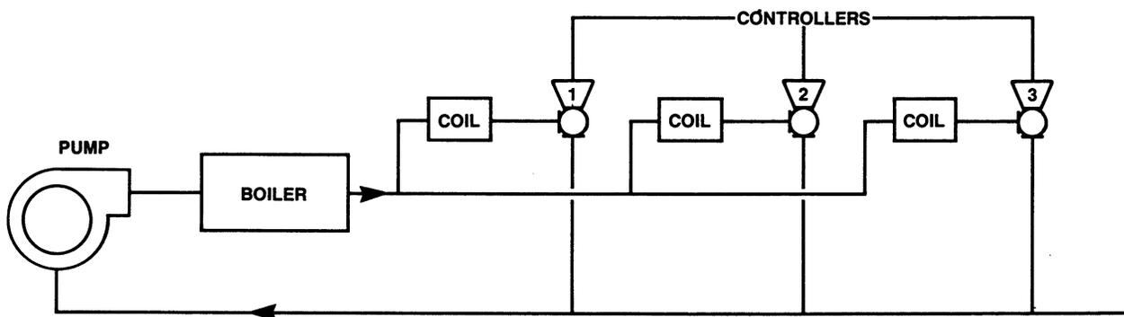
FLOW CONTROL USING TWO-WAY VALVES
