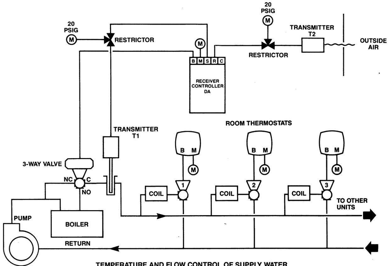
TEMPERATURE AND FLOW CONTROL OF SUPPLY WATER
