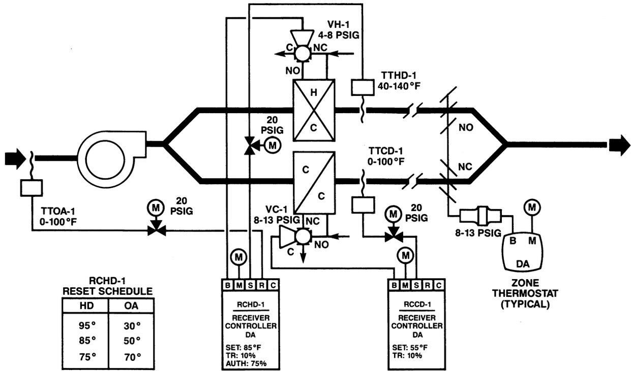
MULTIZONE HOT AND COLD DECK CONTROL WITH HOT DECK RESET
