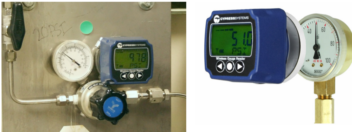
Figure 2 – Non-Invasive Mounting for Wireless Gauge Reader
