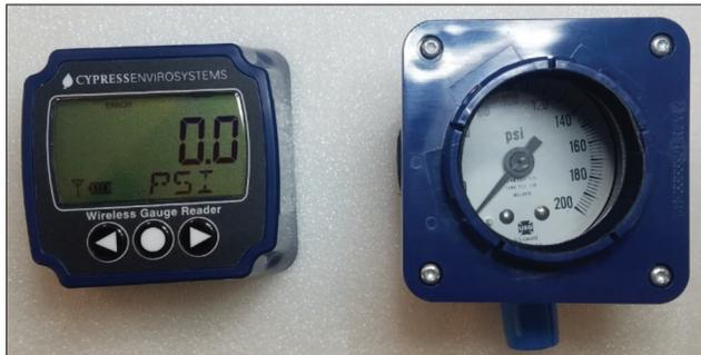
Figure 8 – Convenient access to gauge through quick-disconnect
