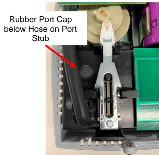
**Figure 17. 2 Pipe Thermostat Port Cap**
