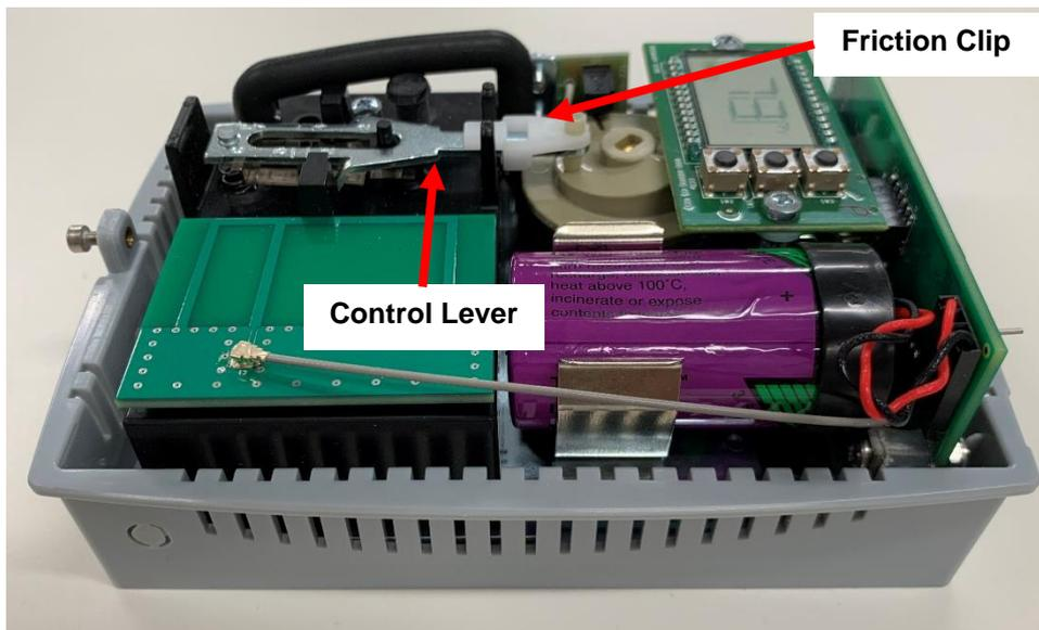
**Figure 15. Friction Clip and Control Lever**
