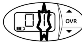
**After entering a correct password, the frequency sub-band will flash signifying Programming Mode**
