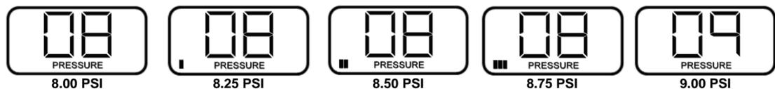
**Figure 13. Pressure Display Resolution**
