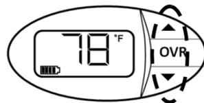
**Press and release all three buttons simultaneously to enter Programming Mode**
