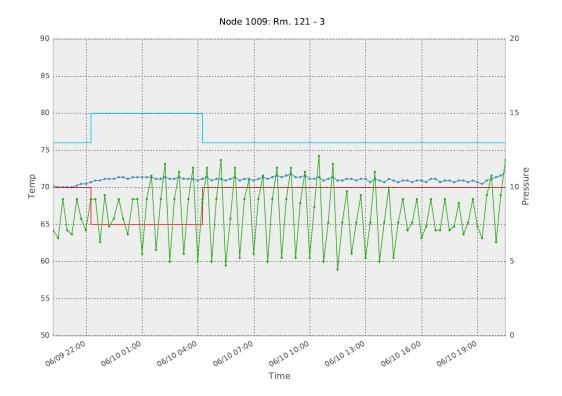
Green Line = Branch Pressure Dark Blue Line = Room Temperature Light Blue Line = Cooling Setpoint Red Line = Heating Setpoint
