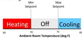
No heating or cooling occurs when the actual room temperature is between the two setpoints. Proper ventilation will continue to work as normal.
